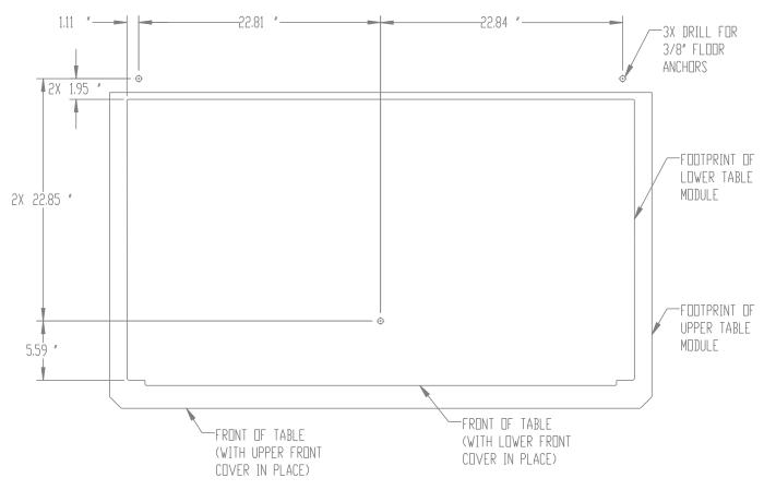
FOR BEST RESULTS, POSITION TABLE AND MOUNTING BRACKETS FIRST AND THEN USE MOUNTING HOLES IN BRACKETS TO DRILL FOR THE FLOOR ANCHORS.
